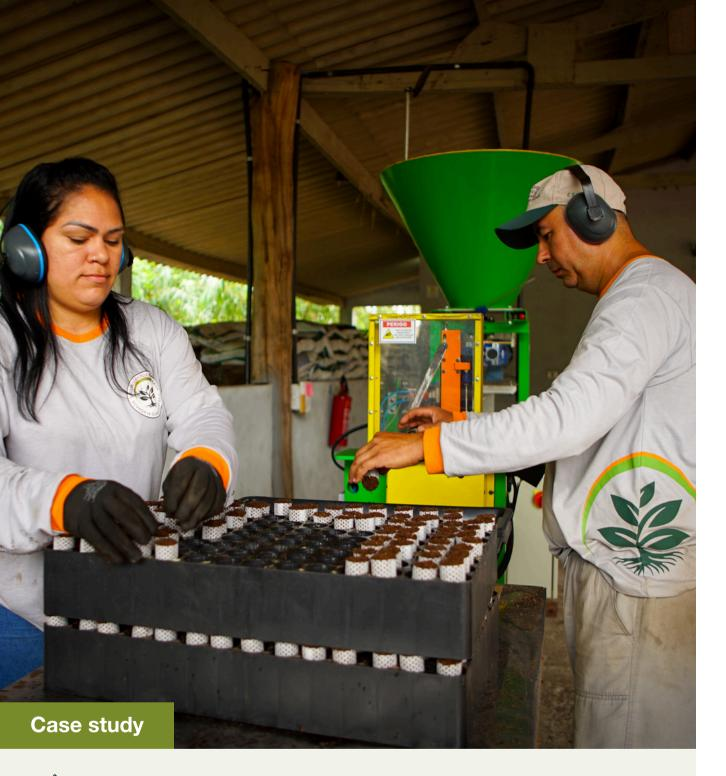
IPÊ's team preparing paper tubes for seedlings using specialized machinery. With this efficient system, they can produce over 12,000 substrate-filled paper tubes—complete with fertilizer—in just three hours. Paper tubes boost forest restoration by providing biodegradable, nutrient-rich containers. Their eco-friendly design eliminates plastic waste and simplifies planting, making them ideal for large-scale reforestation.
